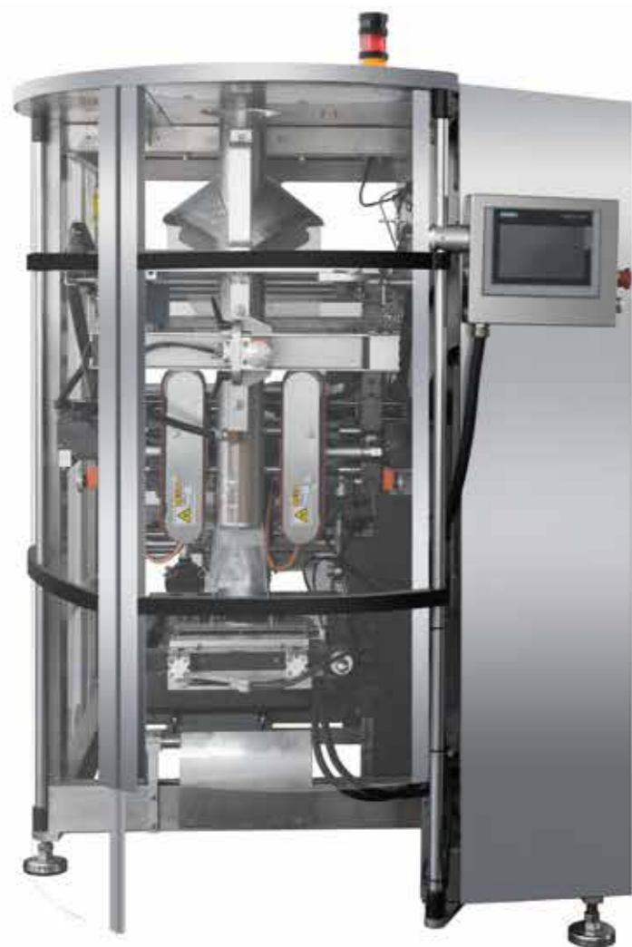
背封连续式立式机(中小袋型/中大袋型) Back sealed, continuous machine (Small bag/Large bag)
